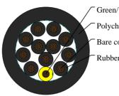
Green/Yellow wire Polychloroprene rubber outer jacket Bare copper conductor Rubber insulation
